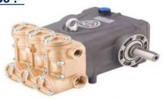
Annovi Reverberi AR RTD130-160 horizontal gas engine triplex plunger pump is rated up to 32 GPM at max 2300 PSI spins a 35mm solid shaft at 1000 RPM using a 1 ½" inlet and 1" discharge thread. N version with a gas engine flange.
